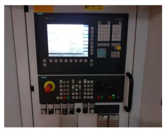
Control Sinumerik 840D Powerline PCU50 HMI Advanced
